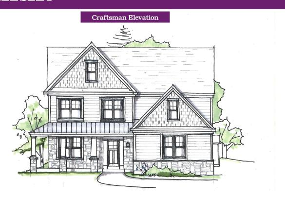
Shown with the following options: wraparound porch with metal roof, stone piers with tapered columns, upgraded front door with surround, pent roof and window in main reverse gable, shake, window, and pent roof in garage reverse gable, and stone water table at garage.
