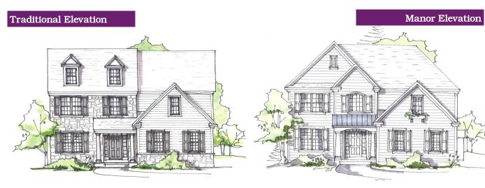
Shown with the following option: 8x8 porch posts, window at garage reverse gable, extended stone front, shutters on foyer window, dormers and stone water table.
